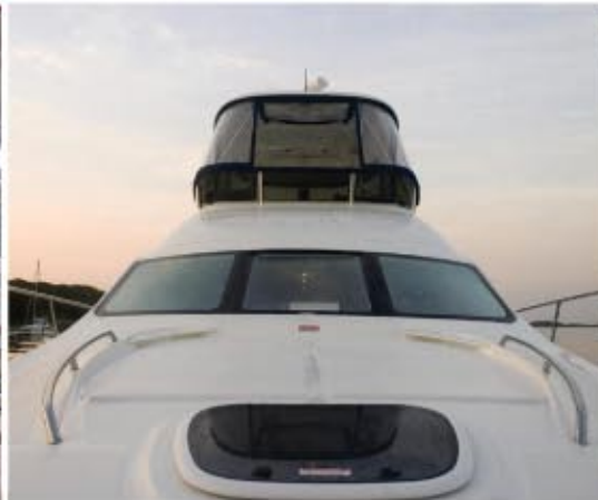
70-08A used for bonding windshields
