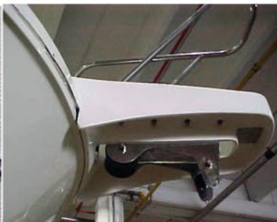
940 FSA can be used as a sealant adhesive to secure pulpit to bow prior to mechanical fastening
