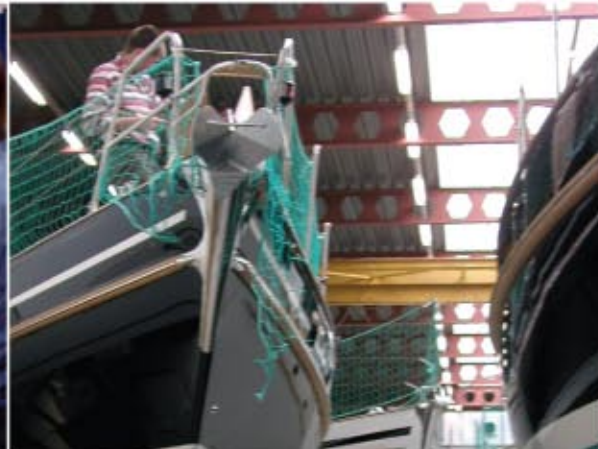
Deck-to-hull bonding with 940 FSA
