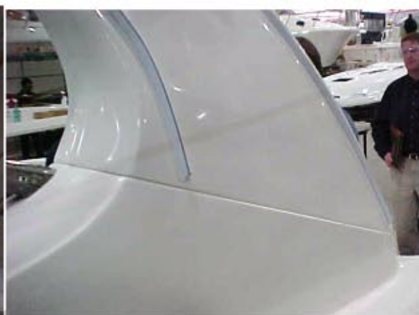
Arch-to-deck joint sealed using 960 SR
