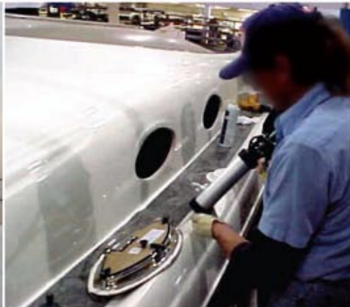
940 FSA used for porthole and hatch installation
